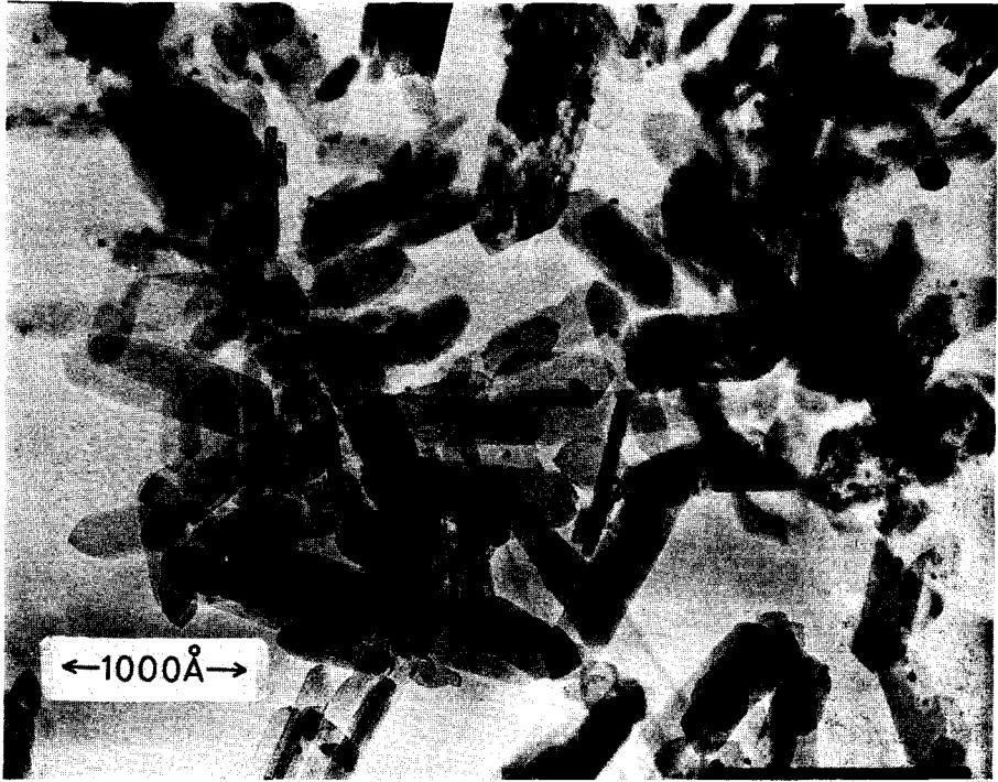
Plate 1. Overall Transmission Electron Micrograph of Standard 32 Å Platinum of Plate-like Alumina.
