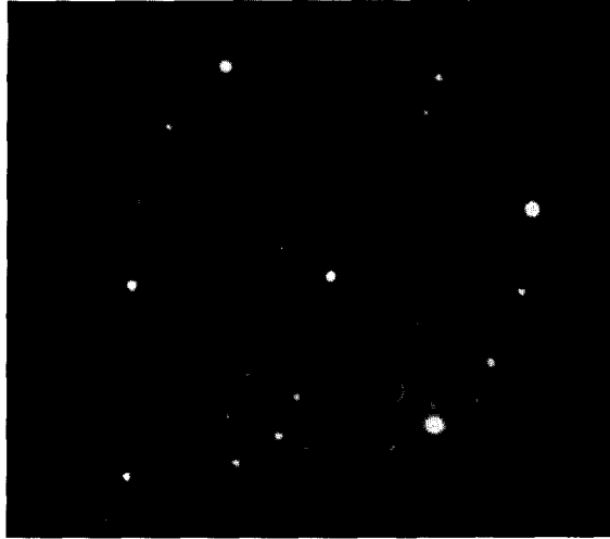
Fig. 2 a. LEED pattern of the \begin{vmatrix} 4 & 0 \\ -1 & 3 \end{vmatrix} and \begin{vmatrix} 3 & -1 \\ 4 & 0 \end{vmatrix} surface structures obtained after heating the \text{NH}_3 covered surface to \sim 520 K (87 eV).
