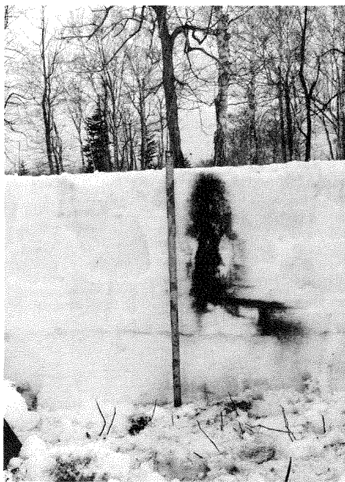
Figure 15 Photograph of dyed meltwater infiltration in a snowpack at the top station on May 7, 1992. The snow depth was 97 cm. There were two ice layers at 50 cm and 38 cm above the bottom.
