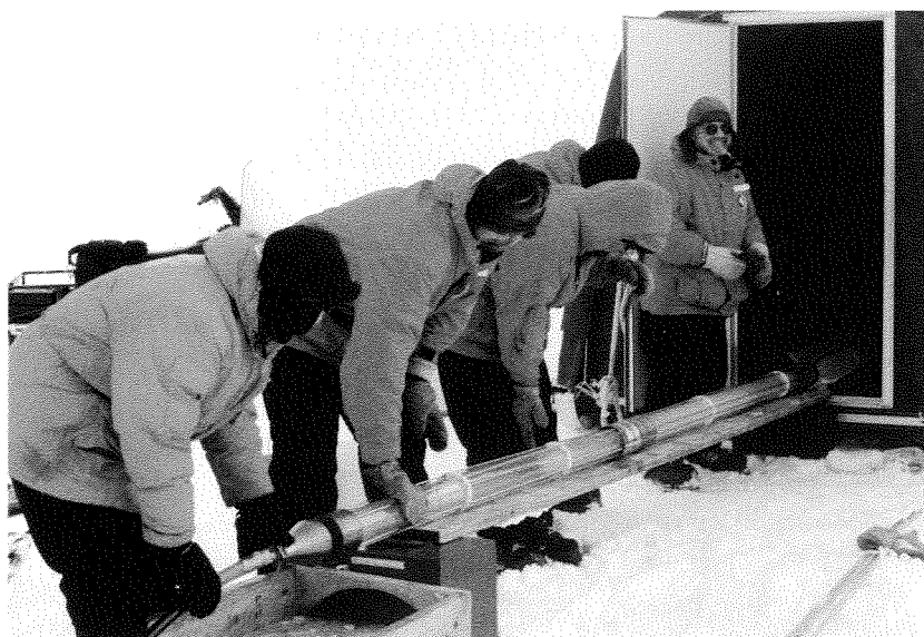
Figure 3: Core being removed from Lexan core barrel used with hot water drill. The barrel is 4 m long and takes a 0.90 – 0.10 m diameter core.
