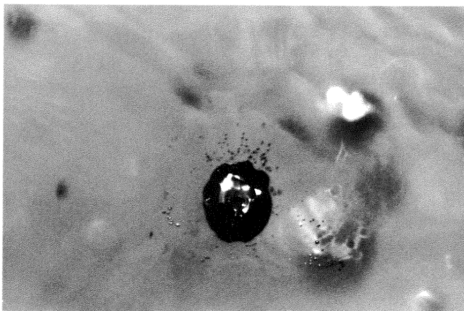
Figure 5: Micro-bubbles surrounding a larger bubble that has grain boundary grooves on its surface. The sample is prepared from a section 1327-m deep in the Summit core. The width of the picture is 2.6 mm.
