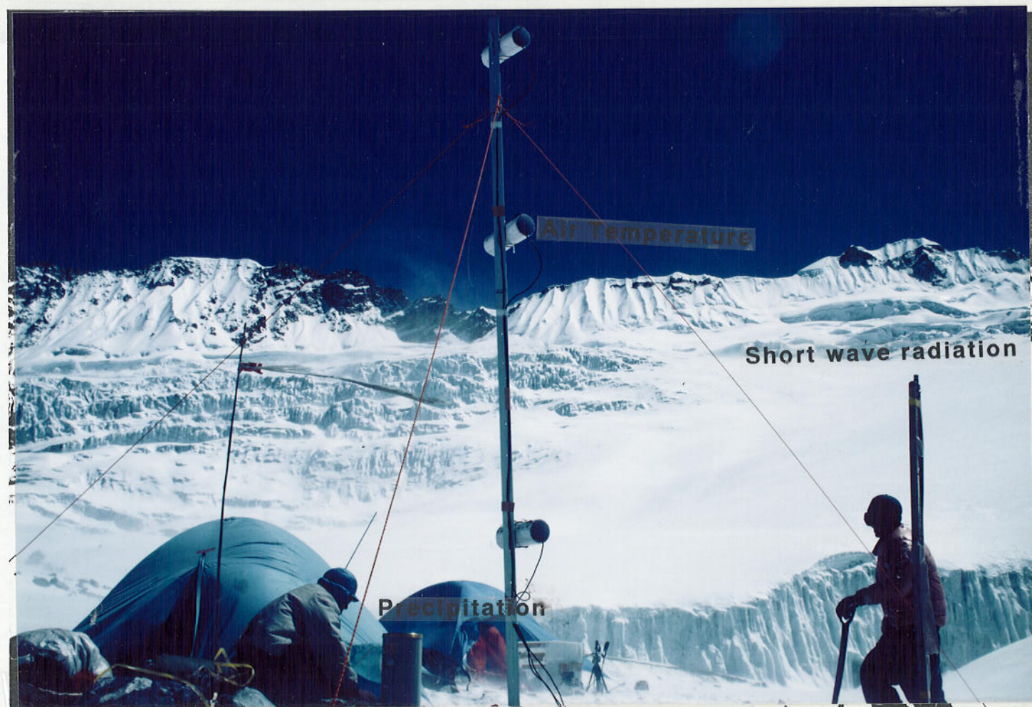
Photo 3.6. The typical meteorological equipments in the forefield of glaciers. This photograph shows the measurements of air temperature, precipitation and short wave radiation at Glacier Camp (GC; 5090 m).
