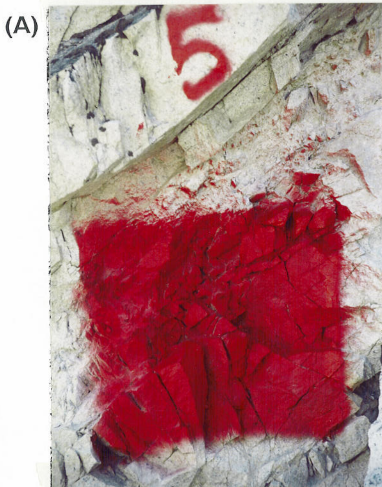
Photo 4.7. A painted rock surface for the measurement of rock breakdown (A: 23 May 1988) and the surface with some fracture one year after the paint (B: 23 May 1989).
