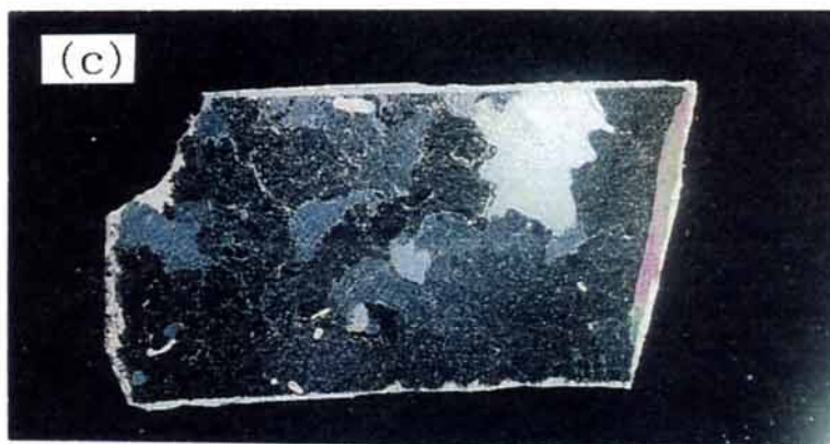
Figure 5.3.11 Polarized photographs of thin section of nilas N2 (1997) taken off the northeastern Hokkaido coast (see Figure 5.1.2c). (a) Full scale sample (b) Vertical section (c) Horizontal section (Black area represents vertical C-axis.)
