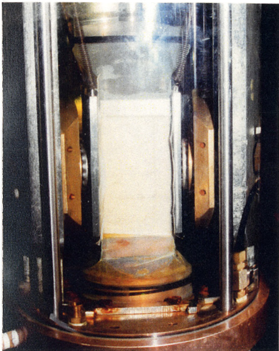
(c) specimen mounted on plane strain test apparatus
