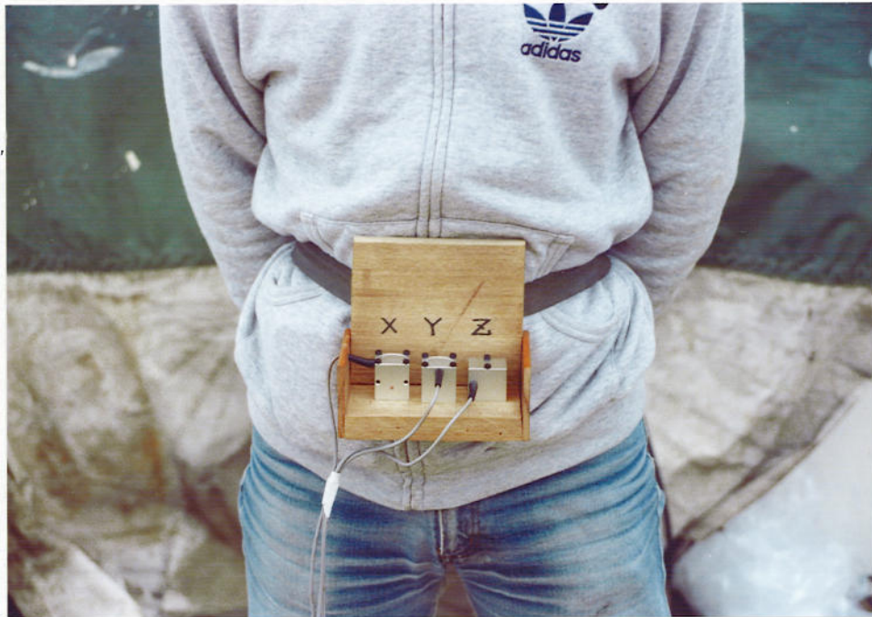
Photo 4-3 View of acceleration measurement device on the subject.
