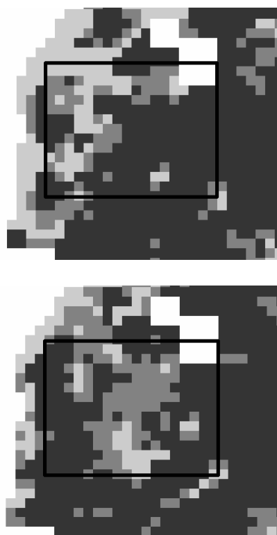
Fig.6.2.5. Height classes analyzed by digital photogrammetry. Upper: Year of 1984, Lower: Year of 1999. Rectangle shows the extent of Fig.6.3.1 Height class; White grid is the exception area. ■:10m ~, □:5~10m, □:~5m
