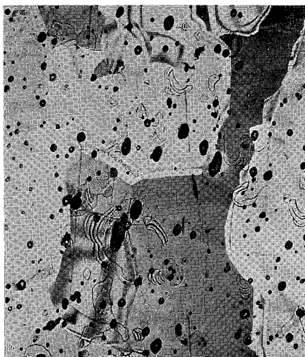
Fig. 5. C1 ice, 680' from the entrance of the tunnel; \rho = 0.911 , \times 7.5 .
