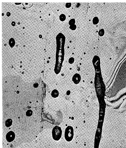
Fig. 4. B2 ice, ice cap ice, \rho = 0.910 , \times 7.7 .
