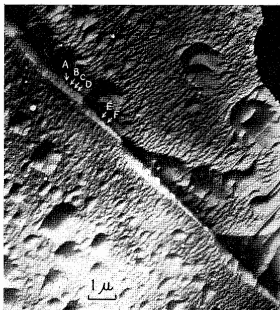
Fig. 6. A row of etch pits at a small angle boundary. Despite of overlapping, each dislocation can be distinguished with its apex as designated by A to F. Electron photomicrograph.
