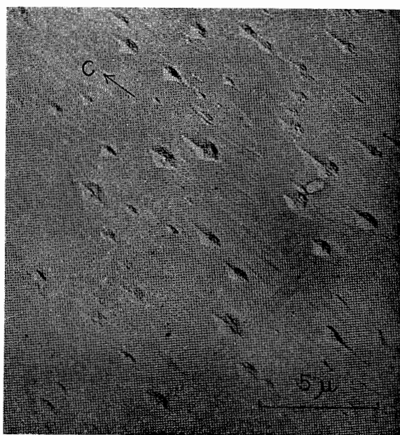
Fig. 2. Etch pits of spindle shape on a prism plane of ice crystal. Electron photomicrograph.
