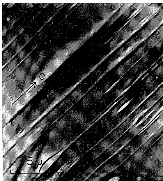
Fig. 4. Further developed stage of spindle shape of etch pits with strong deformation. Electron photomicrograph.
