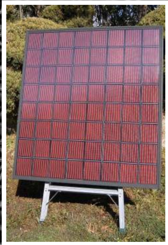
Series connected 64 DSC cells
