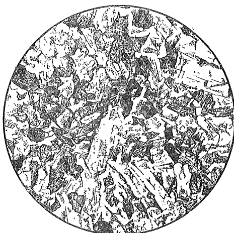
Fig. 6. Hornblende diabase dike cutting the Hikami granite. Middle part between Mt. Hikami and Takata city. Diam. 4mm. Partly ophitic aggregation of andesine, hornblende and opaque minerals.
