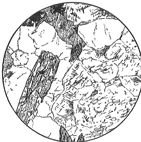
Fig. 3. Acid plutonic rock of the Kesengawa type. Eastern margin of the Tsubosawa Valley. Diam. 4mm. Granodioritic rock containing euhedral plagioclase, green hornblende and biotite with interfilling quartz and orthoclase.
