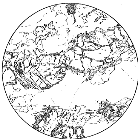
Fig. 11. Cordierite, andalusite gneiss in the Tsubosawa gneiss. North of the Tsubosawa Valley. Diam. 1.5 mm. Cordierite surrounded with yellowish chlorite, which mingles with sericite, and euhedral andalusite: groundmass is mainly composed of quartz and plagioclase.
