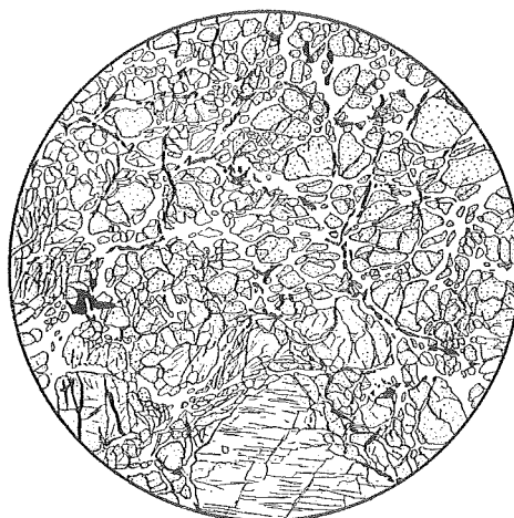
Fig. 4. Serpentinite. Yamabe district. Minute antigorite and chrysotile flakes enclose fresh grains of olivine and clino-pyroxene showing mesh structure. Granules of fine iron ore show the boundaries of the original crystals.
