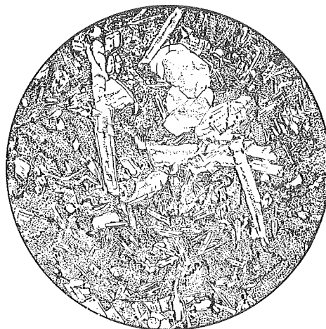
Fig. 8. Diabasic pillow lava. Locality ditto. The rock from the marginal part of the same pillow body showing in Fig. 7, is porphyritic and more or less glassy.
