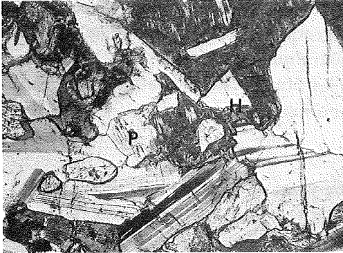
Fig. 33 Mottled part of pyroxene gabbro with clinopyroxene(P) and brown hornblende(H). (partly crossed nicols)
