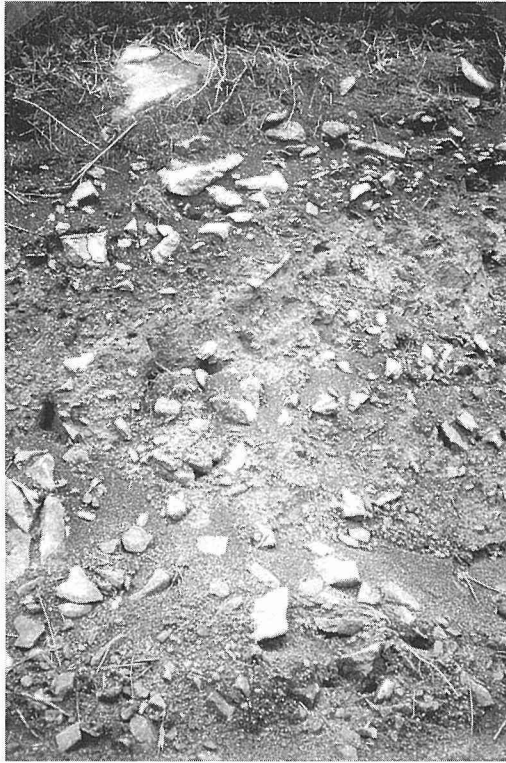
Photo. 10 Section at Loc. 8. Angular gravels are mixed in Kuroboku soil, which is about 25 cm in thickness.
