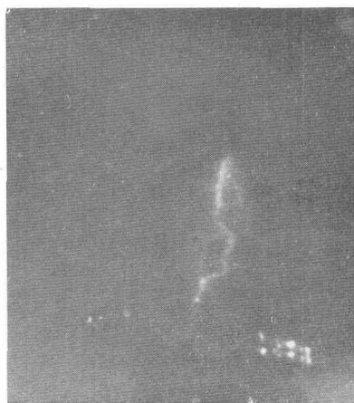
Fig. 122. Streamer in quartz. (magnification 30)
