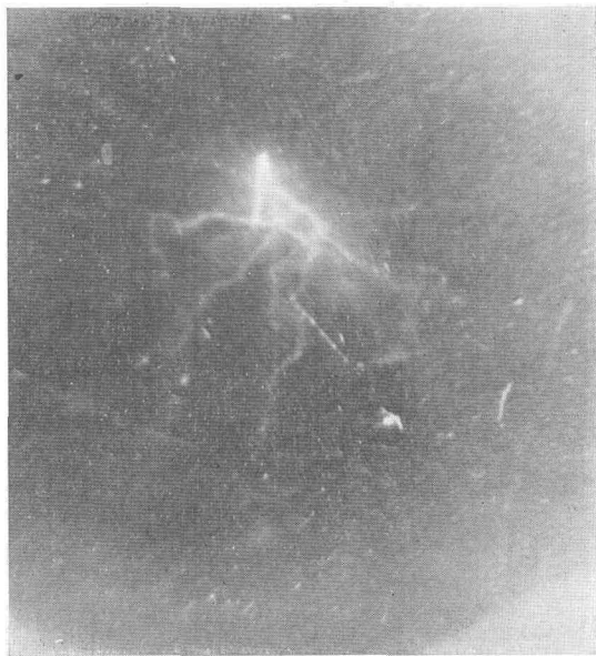
Fig. 18. Streamer in tartaric acid. (magnification 30)
