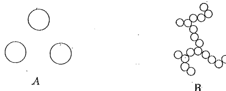
Fig. 4. Schematic representation of two types of colloidal silica particles.
