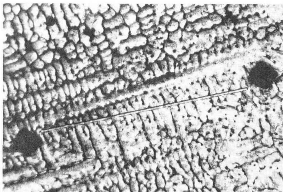
(a) \Delta T = 8^{\circ}\text{C} ; usual dendritic structure
