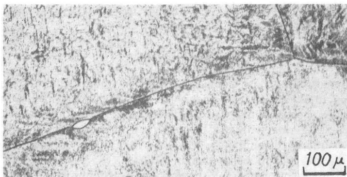
Photo. 1. Dislocation pile-ups along grain boundary produced by cold rolling. Aged at 200°C for 10 hr and etched with Morris etchant.
