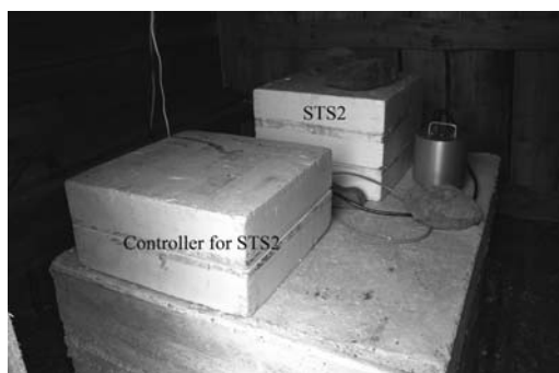
Photo-3. Broadband seismometer at station OHT is covered by a container made of styrofoam.
