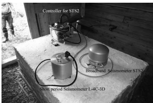
Photo-2. Broadband seismometer STS2 and short period seismometer L-4C-3D at station OHT.
