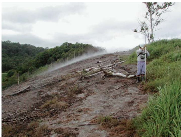
Fig. 1. Measurement of total magnetic field with a proton magnetometer in the western geothermal area.
