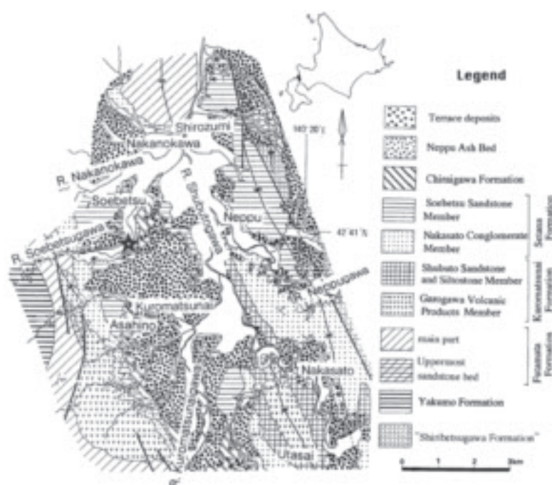
Fig. 1 Geological divisions of the area in and around Kuromatsunai, adapted from [3]. The star indicates the location of the Soebetsu outcrop that exposes the upper part of the Setana Formation and the Chiraigawa Formation. The Setana Formation consists mainly of fine sandstone, with abundant molluscan fossils, nanofossils, and fossil bryozoans.
