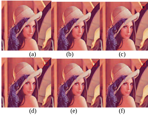
Figure 13 :Error concealment for Lena(512×512). (a)Original (b)With data hiding (53.16db) (c) A MB loss in the image of (b) (d)BI (48.62db) for the image of (c) (e)DI (47.59db) for the image of (c) (f)EX (51.70db) for the image of (c).
