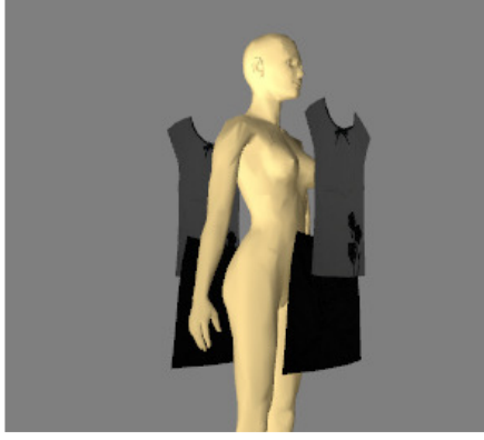
Fig. 7 The front garment mesh is eventually placed in front of the human model, while the back garment mesh is placed in back of the human model
