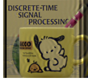
Fig. 6. Reconstructed images from the center of the stereo cameras with 16 [mm] baseline (the difference of disparities become d_1 - d_2 = 14.2 [pixel])
