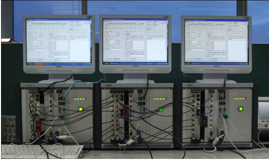
Fig. 2. Transmitter, channel emulator and receiver systems each consisting of a Koden E-1071 signal processing platform.
