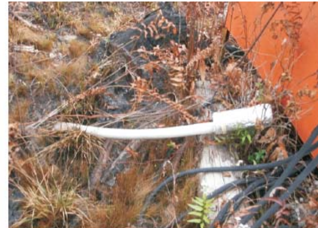
Fig 47. All of cable for gasses measurement was burned (Japanese tower, 05.10.09)
