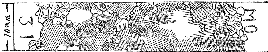
Fig. 2 Stirrated structure of a specimen (No. 31), which was quenched from 530° into water and tempered at 265° for 2 hrs.
