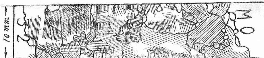
Fig. 3 Striated structure of specimen (No. 32). Its heat-treatment is the same as No.31.
