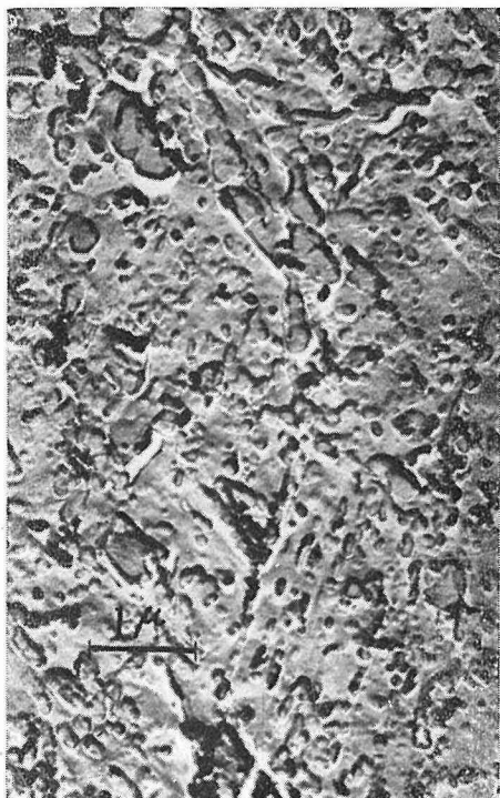
Phot. 5. C 0.28%, Mn 1.39%, Cr 1.95%, Specimen No. 34. \times 12500
