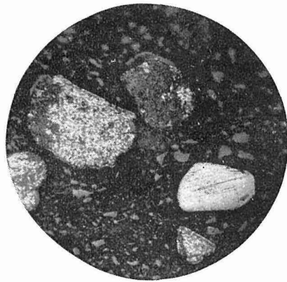
Fig. 2 Roasted product obtained by reducing non-magnetic portion of waste sands from Kunnui in \text{H}_2 gas at 800^{\circ}\text{C} for 1 hr.
