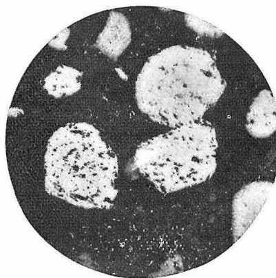
Fig. 6 Roasted product obtained by heating magnetite from Kun-nui in air at 1150°C for 1 hr.
