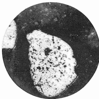
Fig. 26 Roasted product obtained by heating ilmenite from Notoro in air at 1000^\circ\text{C} for 1 hr.
