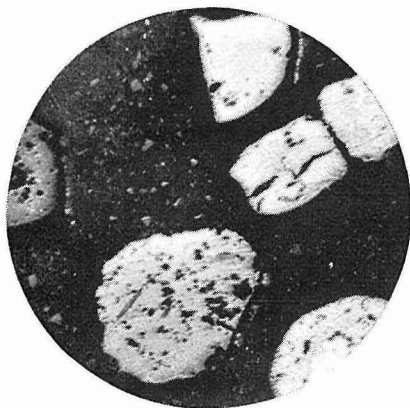
Fig. 25 Roasted product obtained by heating ilmenite from Notoro in air at 900^\circ\text{C} for 1 hr.
