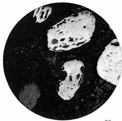
Fig. 20 Roasted product obtained by heating ilmenite from Ōmu in air at 800°C for 1 hr.
