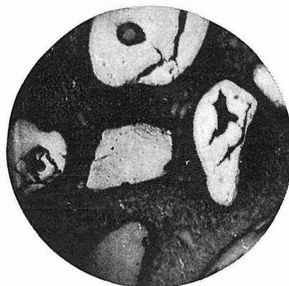
Fig. 37 Roasted product obtained by heating ilmenite from Notoro in air at 900^{\circ}\text{C} for 1 hr.
