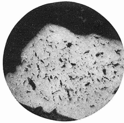
Fig. 22 Roasted product obtained by heating ilmenite from Ōmu in air at 1000°C for 1 hr.
