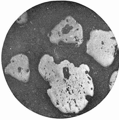
Fig. 1-7. Magnetite from Shirikishinai. Sample was etched with conc. HCl for 20 sec. \times 80
