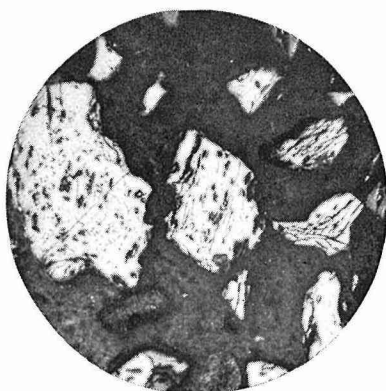
Fig. 12-4. Roasted product obtained by heating magnetite from Kunui in vacuum at 900^\circ C for 1 hr. \times 80
