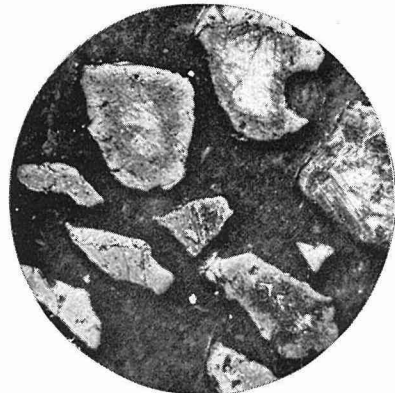
Fig. 18-2. Roasted product obtained by heating synthesized ulvöspinel in air at 600°C for 1 hr. × 80
