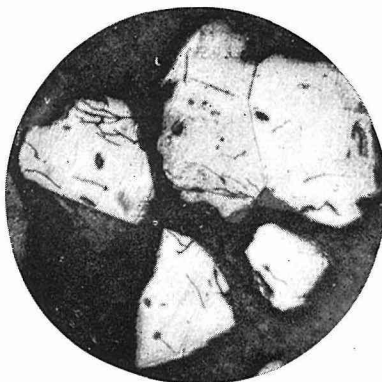
Fig. 12-3. Roasted product obtained by heating magnetite from Kunui in vacuum at 800^\circ C for 1 hr. \times 120
