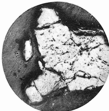
Fig. 19-2. Roasted product obtained by heating titanomagnetite in air at 700°C for 1 hr. × 80
