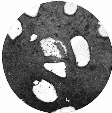
Fig. 2. Magnetite from Kunnui. Sample was etched with conc. HCl for 20 sec. \times 80
