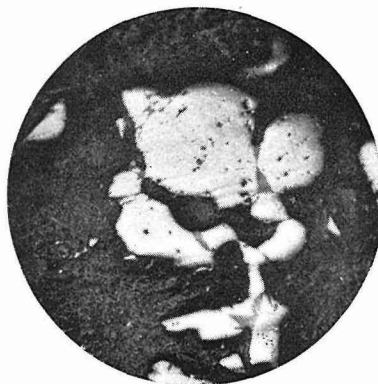
Fig. 12-2. Roasted product obtained by heating magnetite from Kunui in N_2 gas at 1100^\circ C for 1 hr. \times 80
