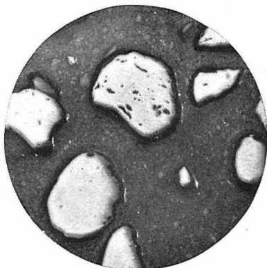
Fig. 1-5. Magnetite from Murooran. Sample was etched with conc. HCl for 20 sec. \times 80
