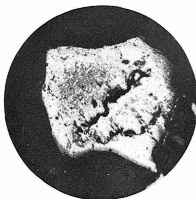
Fig. 19-4. Roasted product obtained by heating titanomagnetite in air at 900°C for 1 hr. × 120
