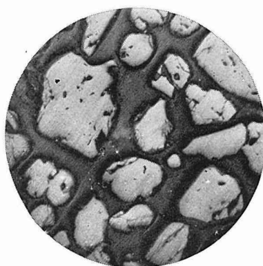
Fig. 12-5. Roasted product obtained by heating magnetite from Kunui in vacuum at 1000^\circ C for 1 hr. \times 80
