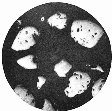
Fig. 12-1. Roasted product obtained by heating magnetite from Kunui in N_2 gas at 900^\circ C for 1 hr. \times 80
