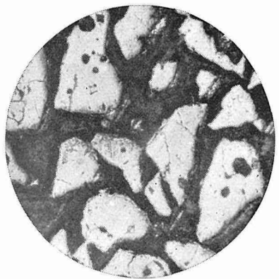
Fig. 18-4. Roasted product obtained by heating synthesized ulvöspinel in air at 800°C for 1 hr. × 80
