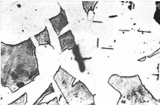
Photo. 3. Microstructure of the specimen of Fig. 3. A trace indicates area in which Fe analyses were made.
