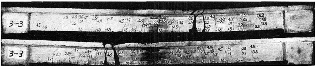
写真 5.17 RC 桁, No. 3-3, P_{cr}=1.50\text{ t} , P_B=5.20\text{ t} , \sigma_{cB}=416\text{ kg/cm}^2 , SS 41 丸鋼
