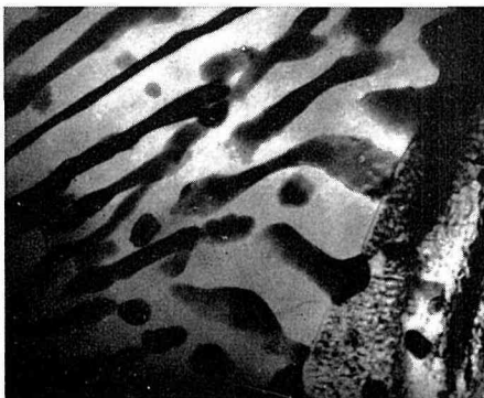
Photo. 10 (c). Aged for 21 min. at 170°C in an electron microscope. Same area as Photo. 10 (a).
