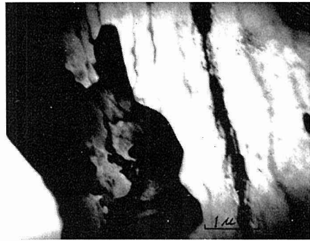
Photo. 11. Preferential precipitation of precipitates on the surface from the foil edge. Aged for 3.5 hrs. at 110°C in an electron microscope. Thin foil was prepared from an as-quenched specimen.
