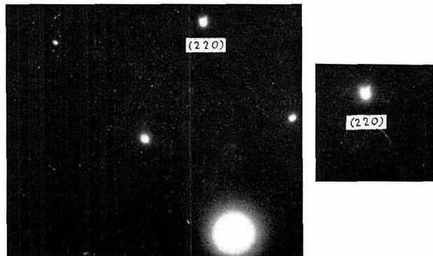
Photo. 7. Electron diffraction pattern after ageing for 8 min. at 175°C. Al-40 wt. % Zn alloy. Same specimen as Photo. 9.
