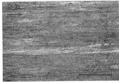
Photo. 1. Optical micrograph of as rolled specimen, showing the band-like structure parallel to the rolling direction.
