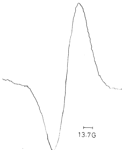
Fig. 10. EPR Spectrum of Trapped Electrons in 2M NaOH Solution 3M rad \gamma -ray Irradiation
