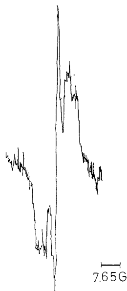
Fig. 11. Resolution Enhanced EPR Spectrum of Trapped Electrons in 2M NaOH Solution 3M Rad \gamma -ray Irradiation
