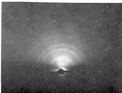
Fig. 6. Reflected electron diffraction pattern of zirconium surface corroded in 10 M \text{NH}_4\text{F} solution
