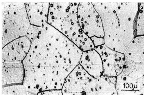
Photo. 1 Microstructure of test piece (Etching: HF-HNO 3 at 20°C for 30 sec)
