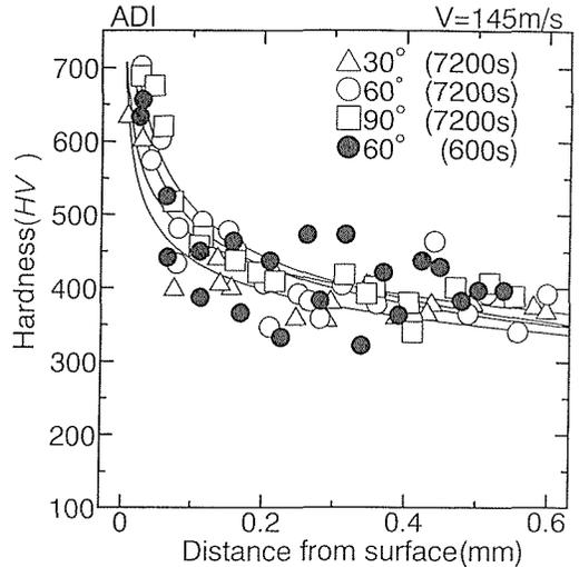
**Figure 11** Hardness (HV) vs. distance from surface, ADI
