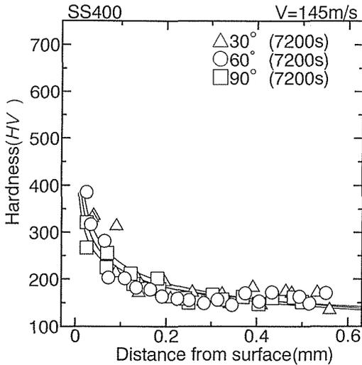
**Figure 10** Hardness (HV) vs. distance from surface, SS400
