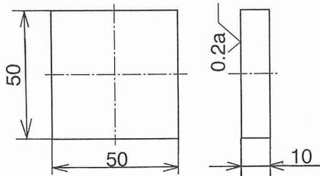
Figure 3 Test specimen
