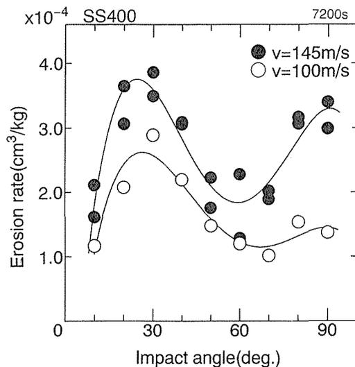
Figure 6 Erosion rate vs. impact angle, SS400
