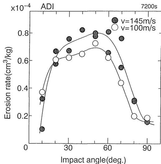
Figure 7 Erosion rate vs. impact angle, ADI
