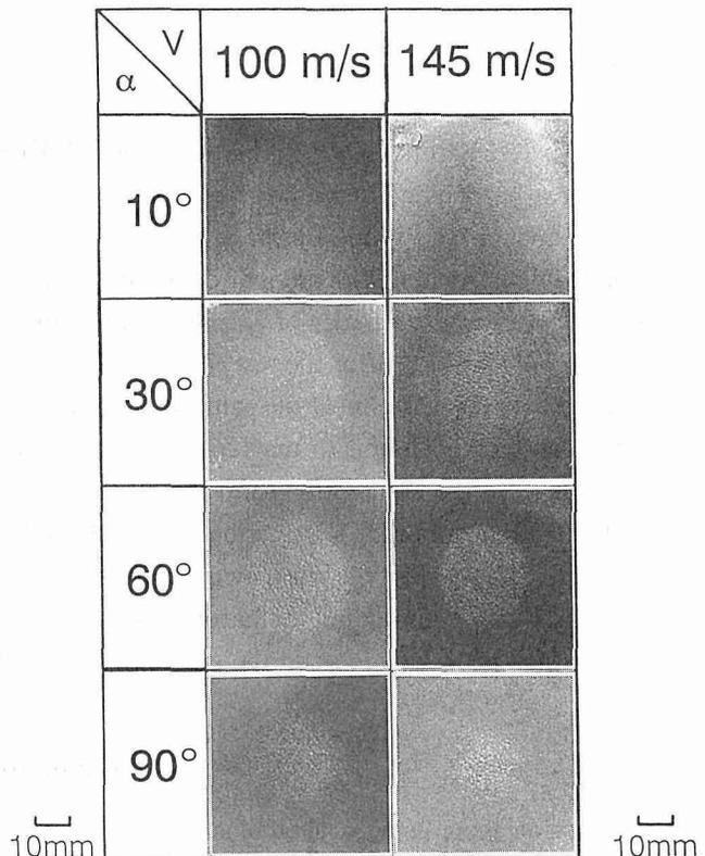
Figure 9 Macroscopic appearance of the eroded ADI surface
