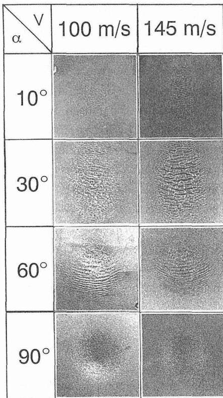
Figure 8 Macroscopic appearance of the eroded SS400 surface
