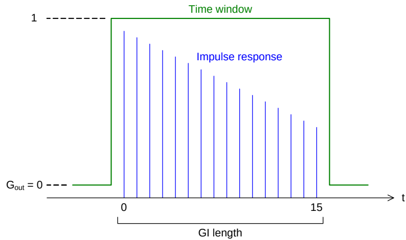
Figure 6.3: Time window function for the conventional SDM.
