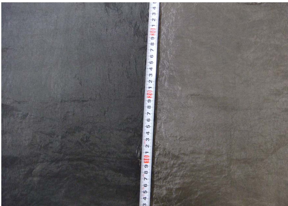
Figure 2 Photos of a section of a typical graphene-coloured fabric (right photo), together with a section of a typical CNT-coloured fabric (left photo).
