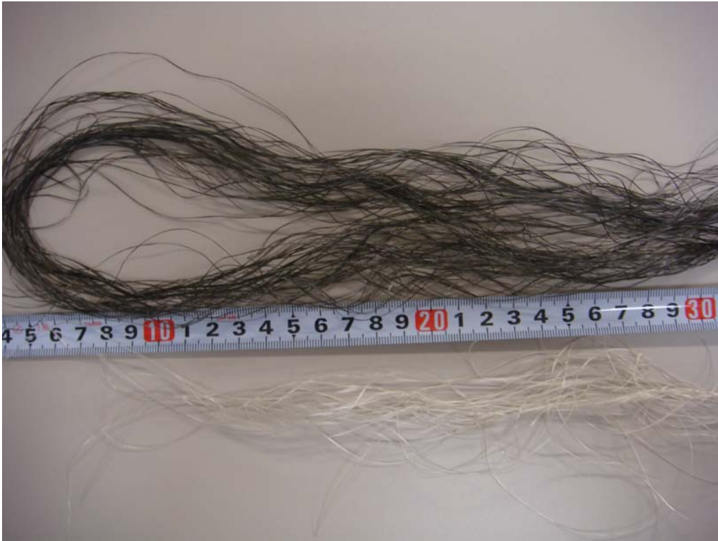
Figure S3 Photos of the graphene-coloured yarn (the dark-black colour) and the pristine yarn obtained by disassembling them from the graphene-coloured fabric and the pristine fabric, respectively.
