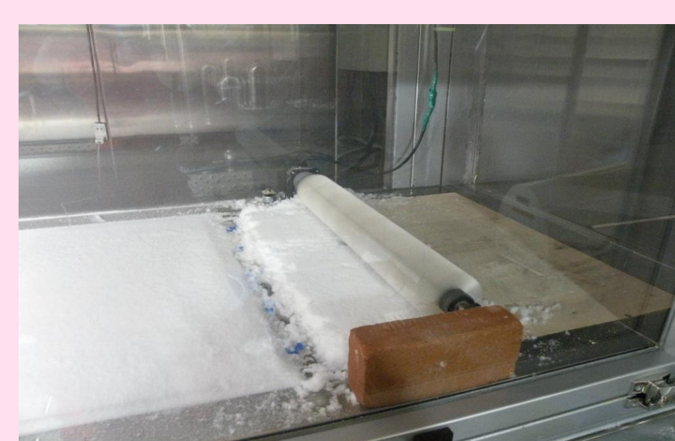
Rolling brush was used to make artificial blowing snow.
