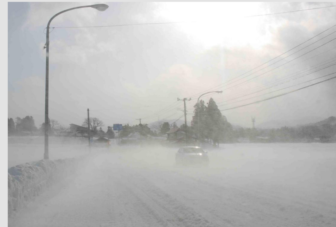
Fig.2 Visibility deterioration Trajectory changing from saltation to suspension causes visibility deterioration.
