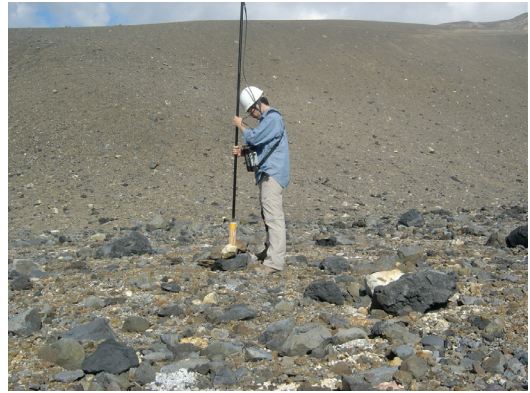
Fig. 1 a. An example of magnetic repeat survey on a wooden peg.
