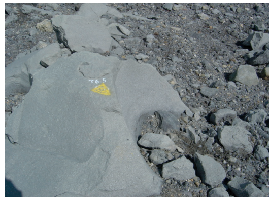
Fig. 1 b. An example of magnetic benchmark on a stable rock.
