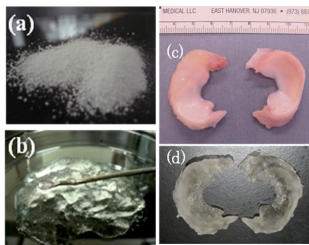
Figure 5 Free shape formation of robust double network hydrogels starting from PAMPS particles (P-DN gel). (a) PAMPS gel particles (powders) in dried state; (b) Swollen PAMPS particles in AAm aqueous solution before gelation; (c) A pair of rabbit meniscus; and (d) artificial meniscus made from P-DN gels.
