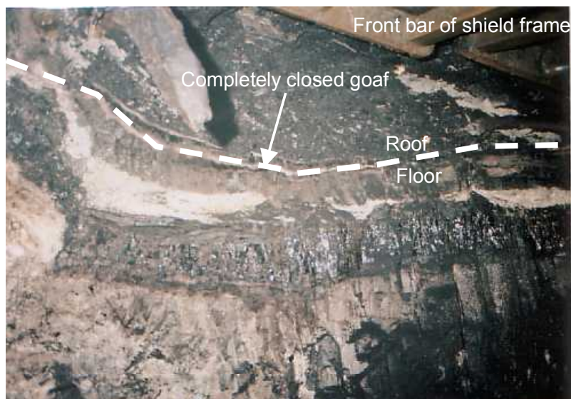
Fig. 15 A goaf of the Main seam mined in 1954, appeared at the working face of Jobu Hidari No.6 SD. The white broken line indicates the boundary between the roof and the floor of the excavated Main seam.
