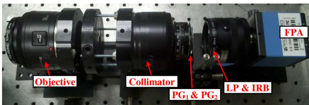
Fig. 7. (Color online) Photo of the CLI polarimeter on the benchtop. This configuration of the polarimeter is optimized for viewing scenes outdoors.
