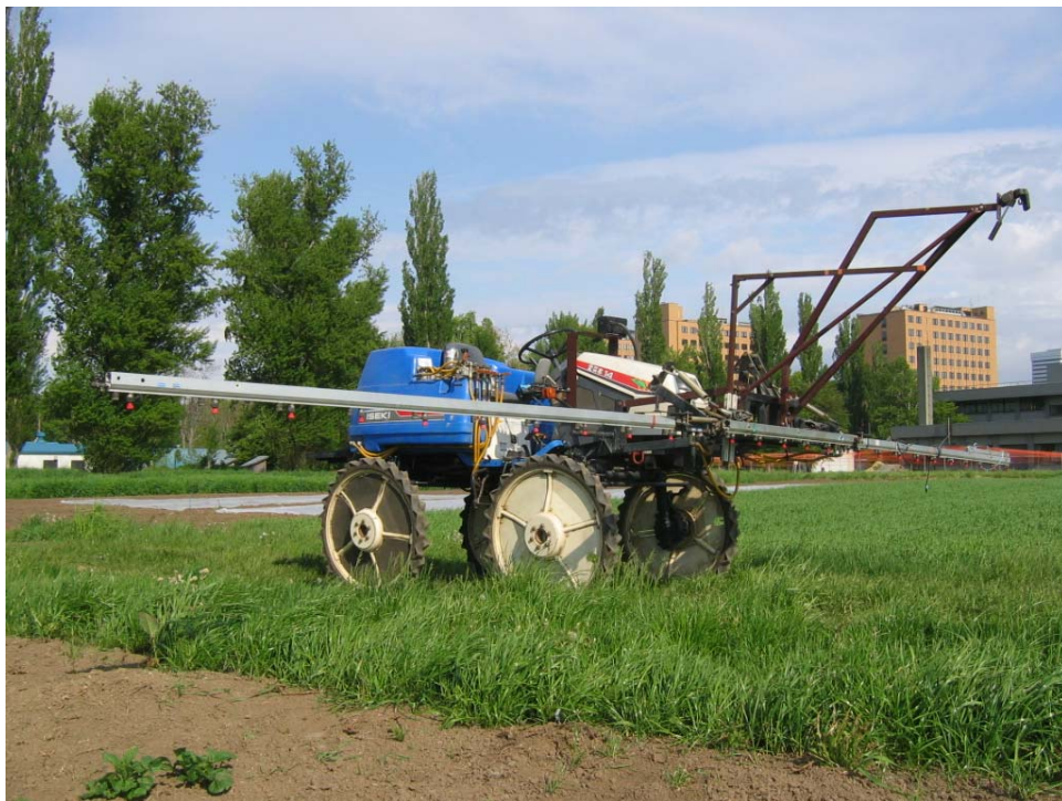
Fig. 6-21. Utility Vehicle (Sprayer Version, Iseki JK-14).
