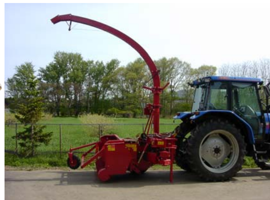
Fig. 6-30. Forage Harvester Mounted on Tractor.
