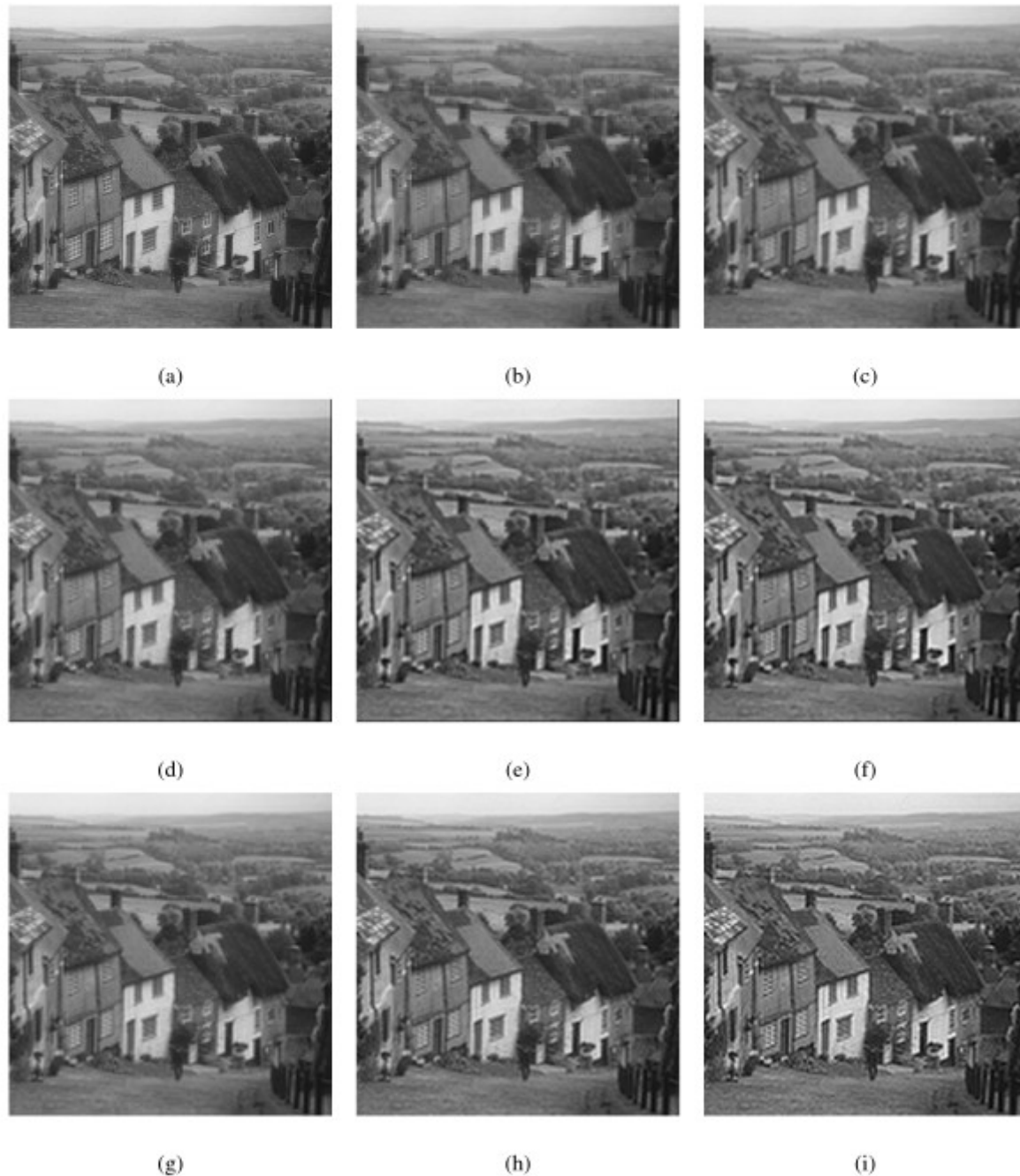
Figure 6 Comparison of results (Test image “Goldhill” (512 × 512 pixels) obtained by using different image enlargement methods. (a) Original HR image. (b) LR image of (a) . HR image reconstructed by (c) sinc interpolation, (d) reference [11], (e) reference [27], (f) reference [8], (g) reference [12], (h) reference [28], and (i) the proposed method.
